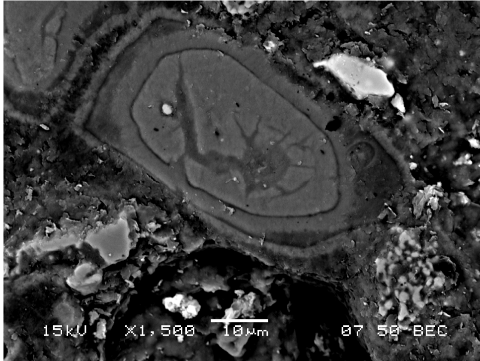
1 2 Figure MgO-4. SEM Image of Premier Chemicals MgO after Hydration in ERDA-6 Brine 3 at 70 °C (158 °F) after 21 days (SNL Experiment CC-ER-70-30-5). Two 4 Concentric Layers of Brucite Surround an Inner Core of Brucite. The 5 Outer Layers of Brucite Appear to be Loosely Attached to the Core.
